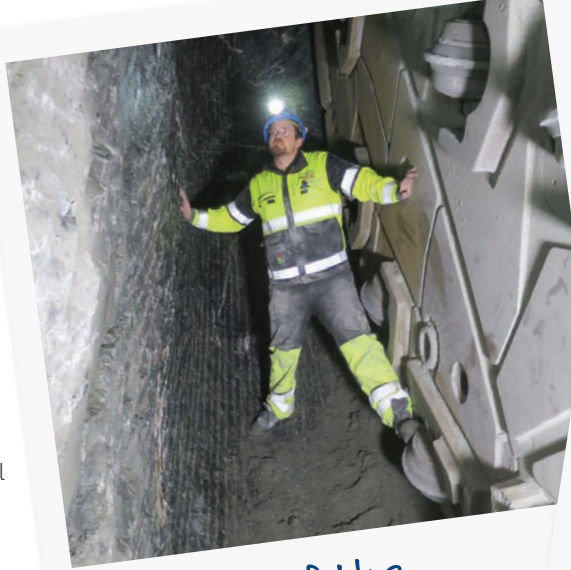
Inspection of the cutterhead
