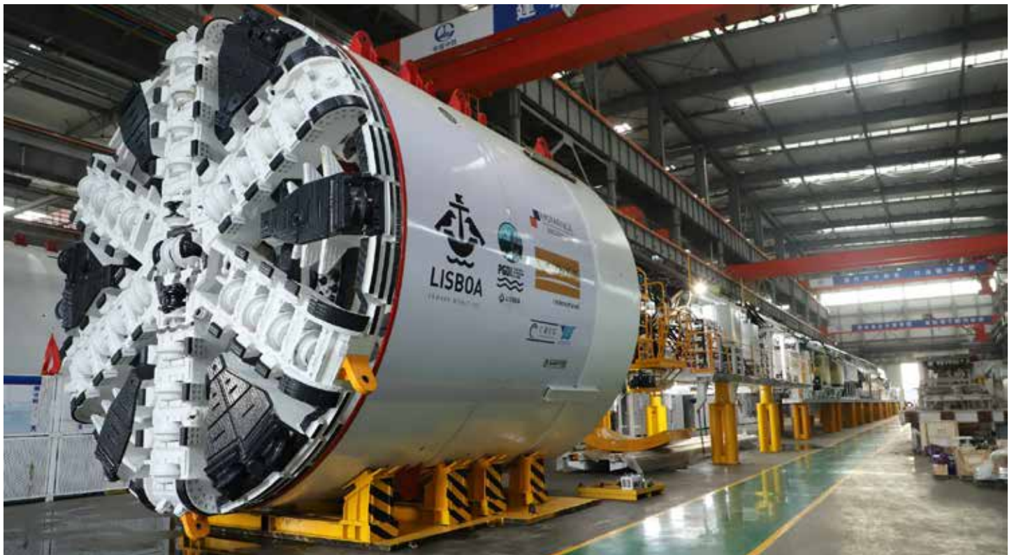
Testing of the TBMs at the factory.
